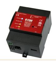
e:cue SYMPL Core S is a stand-alone engine for e:cue SYMPHO-LIGHT with SYMPL Nodes as interfaces. It executes SYMPHO-LIGHT shows in small to medium-sized shows and controls all available SYMPL Nodes. As a user interface it utilizes the Action Pad of SYMPHOLIGHT with all usual web browsers. The connection between Core S, external systems and the Nodes is a standard Ethernet network. Shows can be transferred to the Core S from a SYMPHOLIGHT server or uploaded from many sources.
